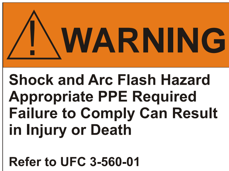
Figure 1-3 Typical Arc Flash Warning Label
