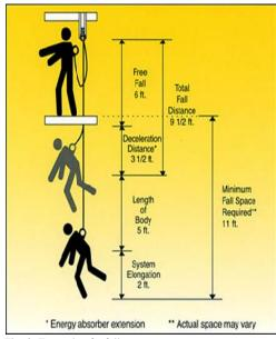
Fig. 3: Example of a fall arrest system
