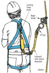
Figure 2: Fall Arrest System
